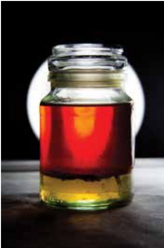
A highly contaminated sample of diesel showing the fuel floating on water with bacterial growth at the interface.
